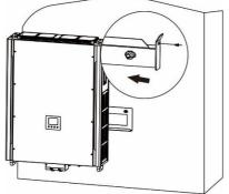
2. Raise the inverter and place it over the mounting plate.
