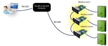
• Use Modbus card to synchronize the parameters:
