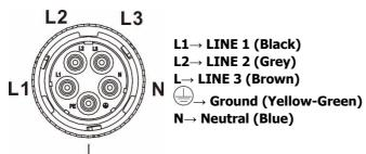
The reference tightening torque is 1.5-2.5 N.m.
