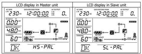
Step 5: If there is no more fault alarm, the parallel system is completely installed. Step 6: Please switch on all breakers of Line wires in load side. This system will start to provide power to the load.
